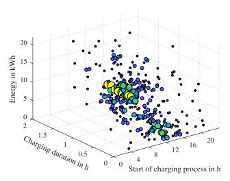
Fig. 4. Load behavior of the fast charging post
