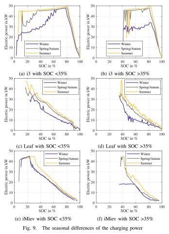
is no range with a constant charging power, consequently this explains the low average charge rating observed in figure 5. Another effect of the temperature can be noted: With a higher start temperature the Leaf is able to receive a noticeably higher power rate throughout the entire charging session. This is particularly notable in winter with a high start SOC, whereby the power rapidly drops into the power ranges of non-fast charging modes 1 and 2 (see figure 9d).
