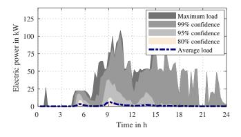
Fig. 7. Load profile of the Fraunhofer fast charging station
